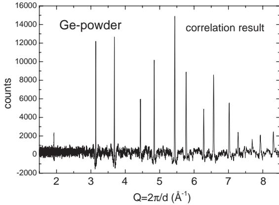
Fig. 2. Data of Fig. 1 analyzed with the correlation method.
