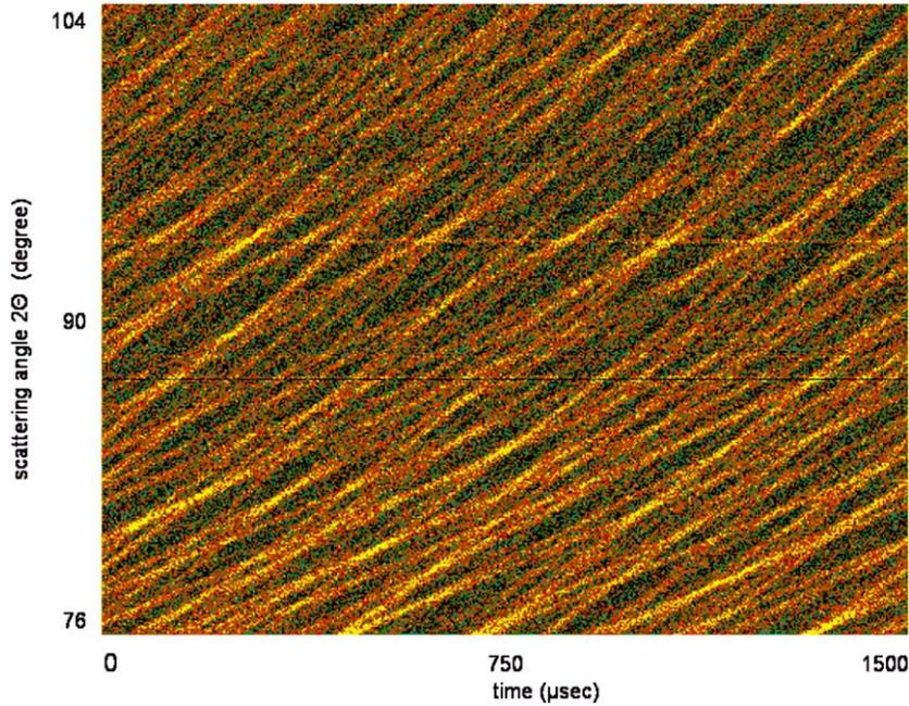
Fig. 1. Raw data of a powdered Ge sample measured on the multiple pulse-overlap diffractometer POLDI. The intensity is color encoded in this plot.
