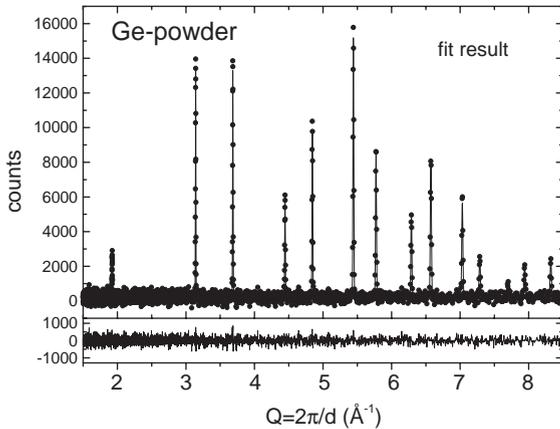
Fig. 4. The fit result of Fig. 3 converted into a diffractogram is shown as solid line. The data points are the sum of fit result plus residuals. The residuals have been calculated from the difference between Figs. 1 and 3 with a correlation method.
