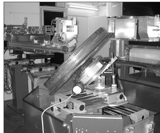
als can be studied in-situ during tensile loading on POLDI. Currently, a 10 kN stress rig is available.
